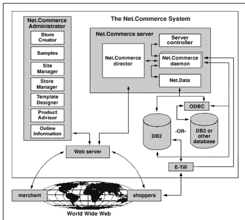
Fig. 2. The IBM Net.Commerce Architecture (Source: IBM)
