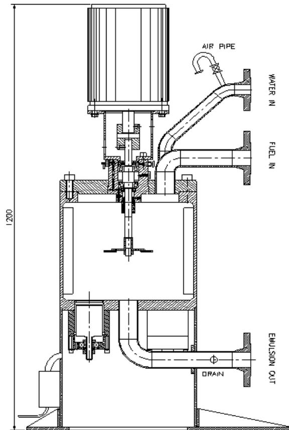
**Figure 2: A schematic profile of the ultrasonic homogenizer**
