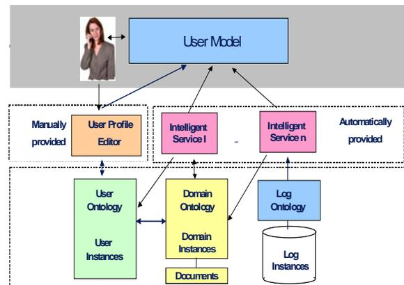
Figure 1: Ontology-based user modeling architecture
